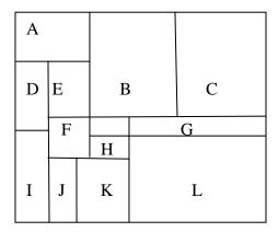
4. Explain Horizontal Virtual Grid Compaction algorithm and apply the algorithm to the given layout and give the compacted layout.
